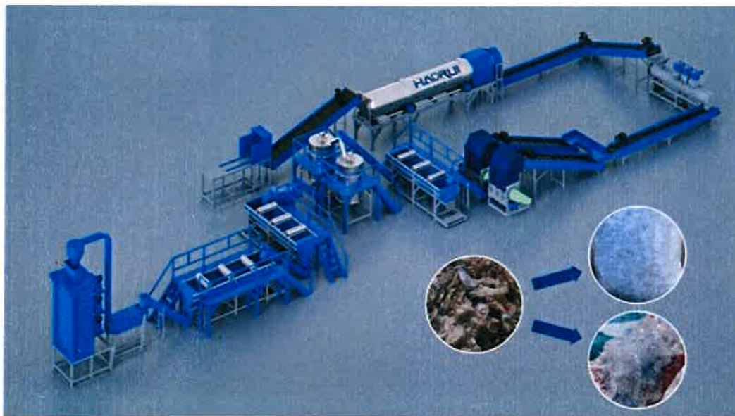
Figure 10. Sample thermomechanical recycling machine line
